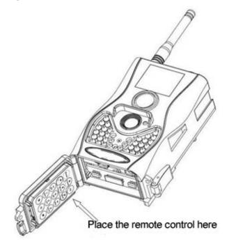
Fig.3 Place for remote control
