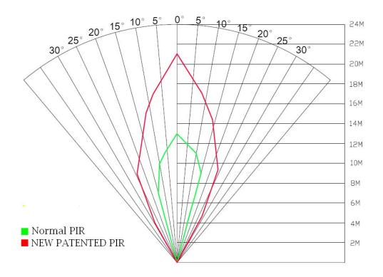
Fig.8 PIR Detection Range
