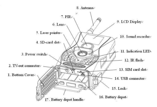
Fig.1 Diagram of camera functional indicators
